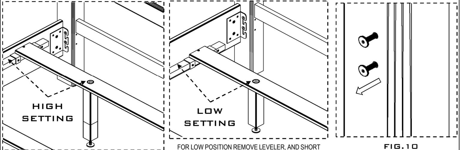
FOR LOW POSITION REMOVE LEVELER, AND SHORT PART OF THE CENTER SUPPORT LEG, THEN INSTALL BACK LEVELER TO THE LONG PART.
