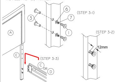
TIGHTEN IN THE CENTER SUPPORT LEG TO THE INSERT NUT
