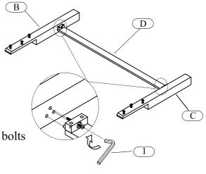
Step 2: Using the Allen key (1) to tighten all bolts
