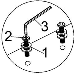
ASSEMBLE HEADBOARD FRAME TO BASE. LOOSELY INSERT ALL 12 BOLTS INTO HEADBOARD, THEN TIGHTEN ALL BOLTS.
