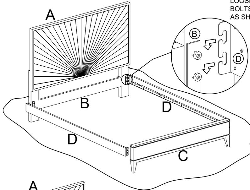
LOOSEN PRE-PARTIALLY TIGHTENED BOLTS, ALIGN SIDERAIL WITH BOLTS AS SHOWN.
