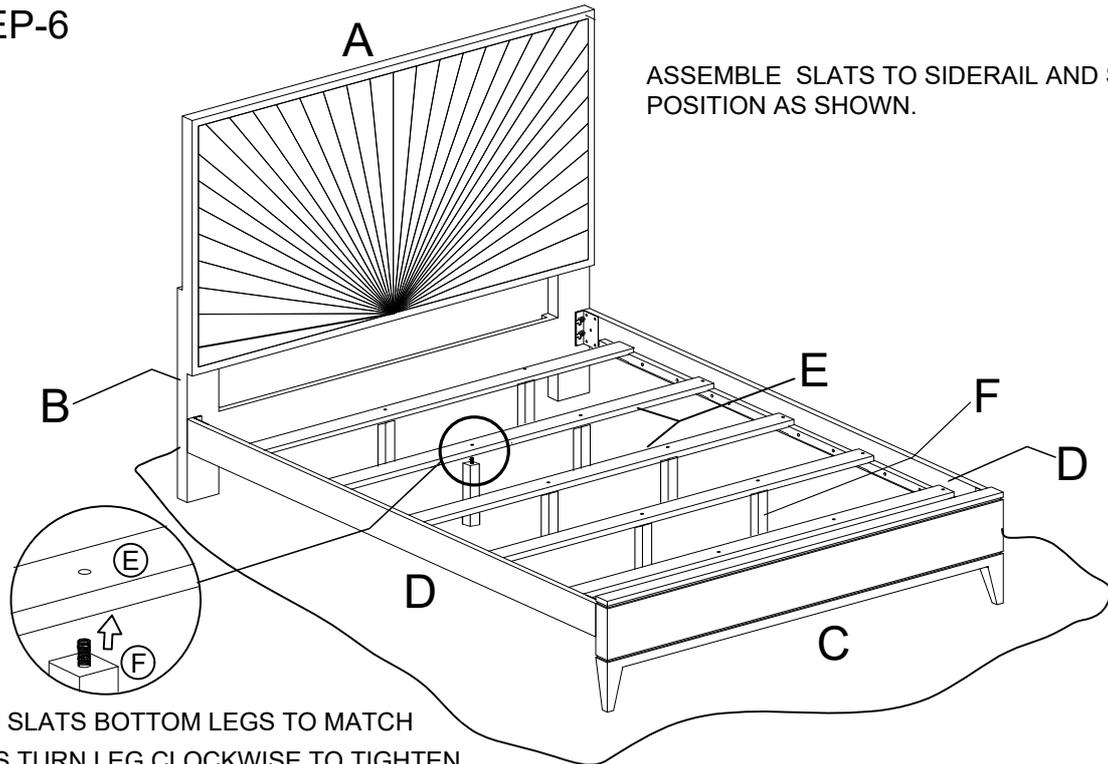
ALIGN SLATS BOTTOM LEGS TO MATCH HOLES TURN LEG CLOCKWISE TO TIGHTEN COMPLETE, REPEAT STEP FOR OTHER LEGS.
