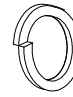
(F) x8 Spring washer * x8 Rondelle a ressort x8 Arandela auto bloqueante
