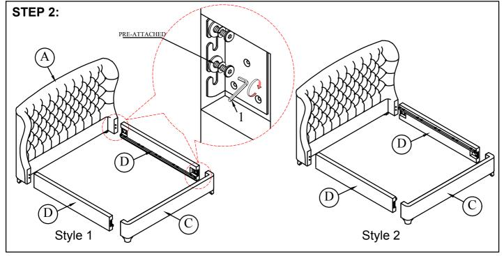
Loosen the Bolts which pre-fixed on Headboard & Footboard.
