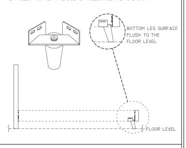
STEP 6 - ATTACHING CENTER SUPPORT LEG TO THE SLAT
