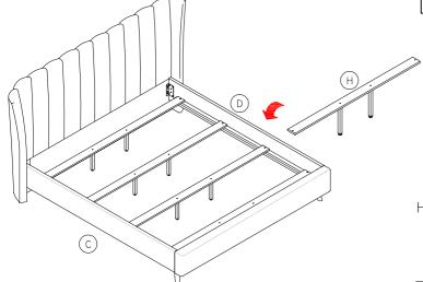
\*NOTE: THE THRU HOLE CAN BE FOUND AT THE MIDDLE OF THE SLAT
