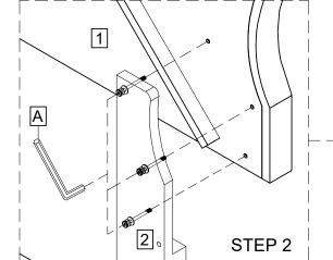
NOTE: The Headboard and Footboard bolts are already pre-installed. STEP 1 : Assembly Stretcher rail (4) with HB legs using allen key (A). Do not tighten all bolts until HB is fully assembly.
