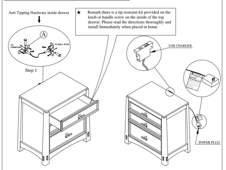
Step 1: Please use a screwdriver (not provided in package) to install the tip restraint kit.
