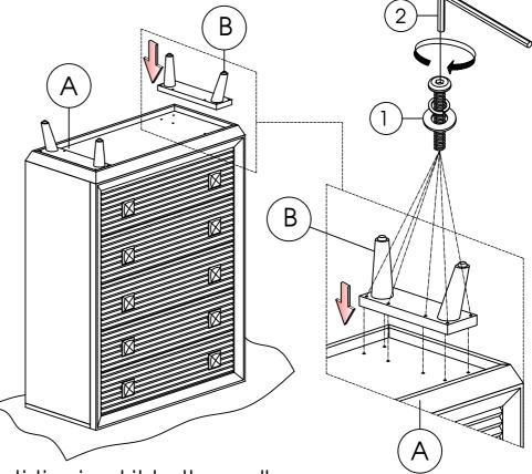
STEP 2 Attached the anti-tipping kit to the wall
