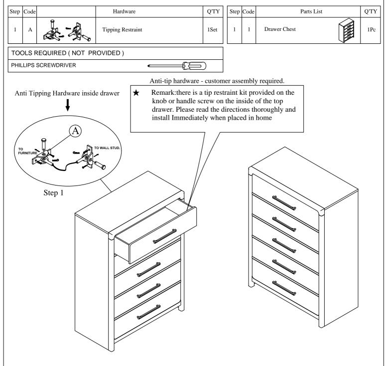
Step 1: Please use a screwdriver (not provided in package) to install the tip restraint kit.
