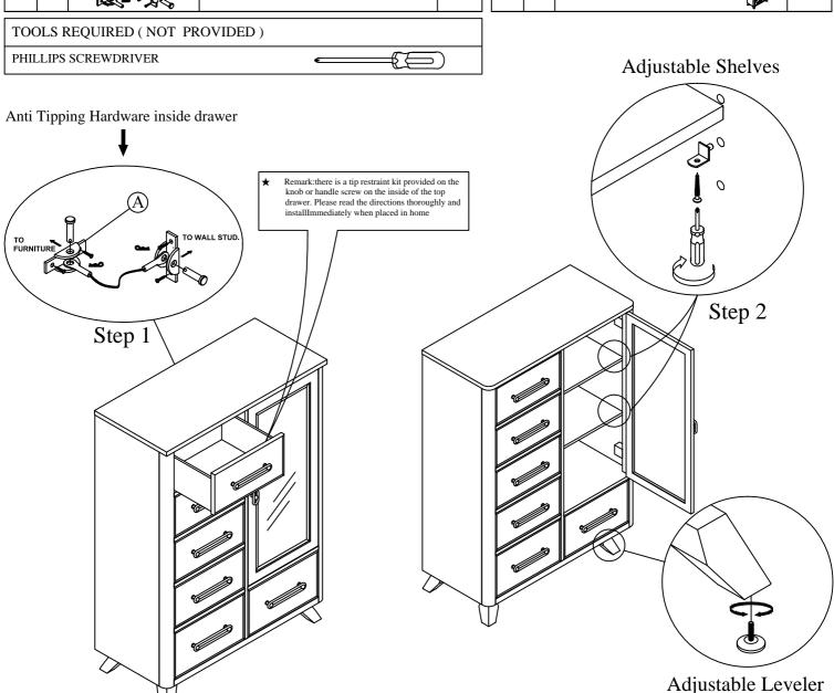
Step 1: Please use a screwdriver (not provided in package) to install the tip restraint kit. Step 2: Please use a screwdriver (not provided in package) to adjust the shelf up or down
