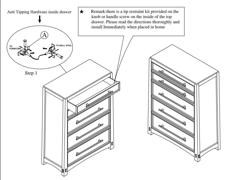
Step 1: Please use a screwdriver (not provided in package) to install the tip restraint kit.
