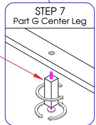
Step 7 . Insert the bolts on the center leg (G) into the pre-drilled holes on the slats (F) secure by turning clockwise.
