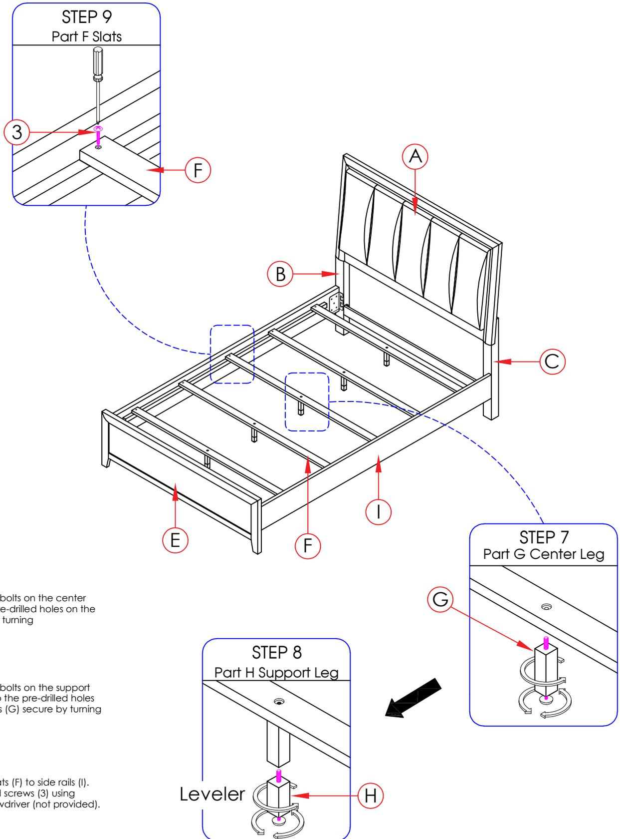
Step 7 . Insert the bolts on the center leg (G) into the pre-drilled holes on the slats (F) secure by turning clockwise.
