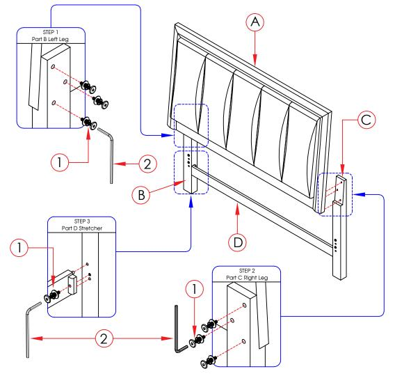
Step 3. Attach the headboard Stretcher (D) to headboard leg and secure with flat washers, lock washers and bolts (1) using allen wrench (2).
