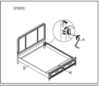
Remove bolts from headboard and footboard then attach side rails to headboard and footboard with the bolts just take off.
