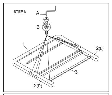
Attach Headboard post to Headboard panel, Assemble Headboard bottom rail to headboard posts.
