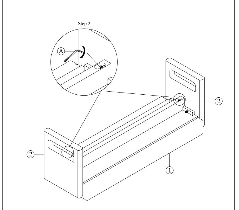
Remark: The bolts were pre-installed on bench cushion. Step 2: Attach bench leg (2) to bench cushion (1) by using allen key (A) tighten the bolts.
