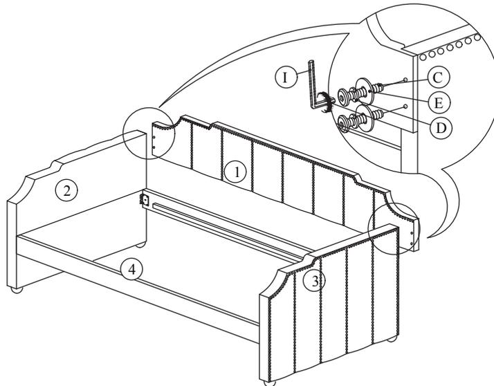
**4** Tighten all bolts from STEP 2 using the Allen Wrench (J) that has been provided. Now only tighten bolts for STEP 3 using Allen Wrench (I). Attach Slat (7) to Front Rail (4) and Back Rail (5) by unrolling and securing with 4 Wood Screws (G) 2 per each side. Tighten all screws using philips head screwdriver (not included)
