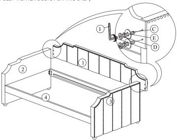
Tighten all bolts from STEP 2 using the Allen Wrench (J) that has been provided. Now only tighten bolts for STE P3 using Allen Wrench (I). Attach Slat (7) to Front Rail (4) and Back Rail (5) by unrolling and securing with 4 Wood Screws (G) 2 per each side. Tighten all screws using philips head screwdriver (not included)
