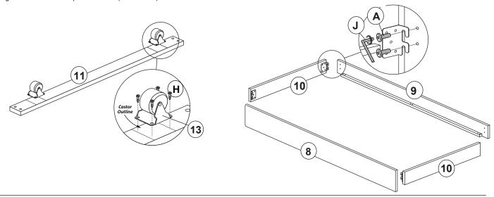
3 Attach Slats (11) to Front Rail (8) and Back Rail (9) using 2 Bolts (B), 2 Spring Washers (D) and 2 Flat Washers (F) on each end of each Slat (11).
