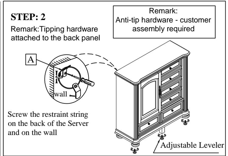
Screw the restraint string on the back of the Server and on the wall
