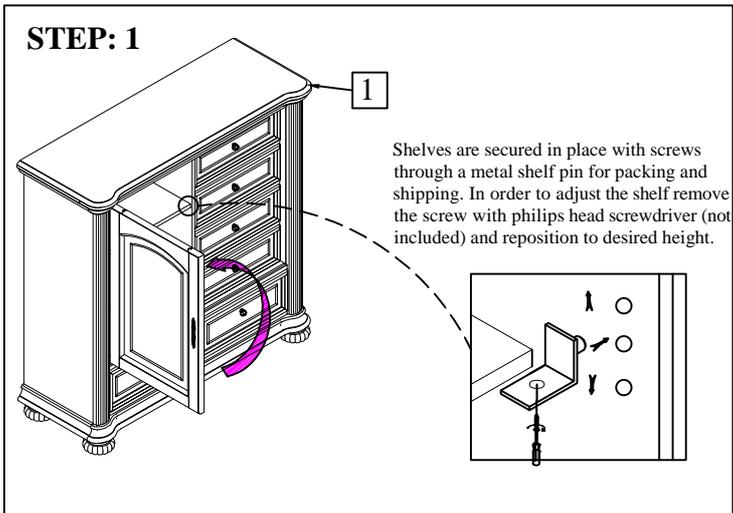
Shelves are secured in place with screws through a metal shelf pin for packing and shipping. In order to adjust the shelf remove the screw with philips head screwdriver (not included) and reposition to desired height.
