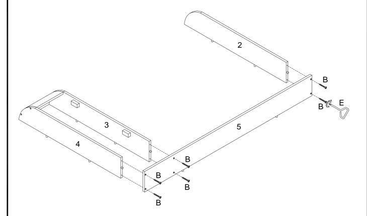
Using screw (B) attach part (5) to parts (2,3,4) with screwdriver (E) as per diagram.
