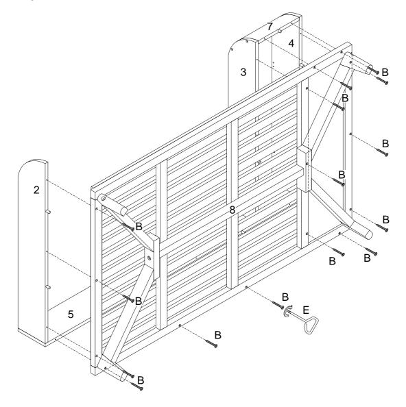
Using screw (B) attach part (8) to parts (2,3,4,5,7) with screwdriver (E) as per diagram.
