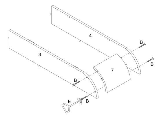
Using screw (B) attach parts (3,4) to part (7) with screwdriver (E) as per diagram.
