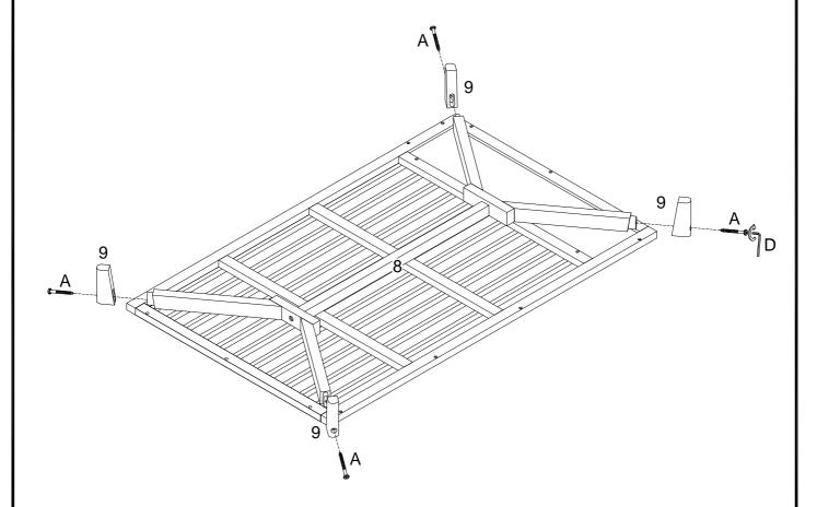
Using screw (A) attach part (9) to part (8) with Hex key (D) as per diagram.
