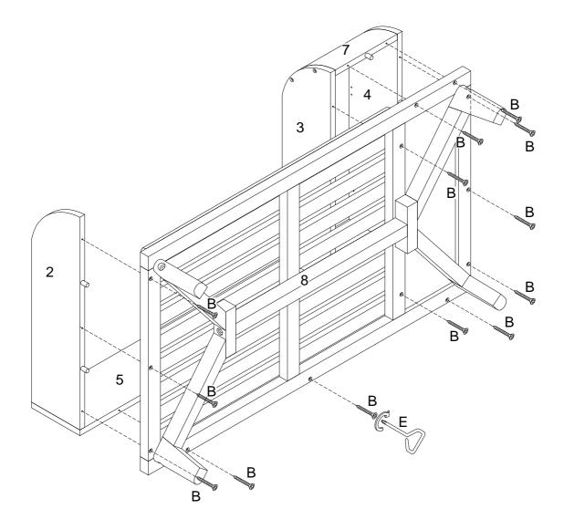
Using screw (B) attach part (8) to parts (2,3,4,5,7) with screwdriver (E) as per diagram.
