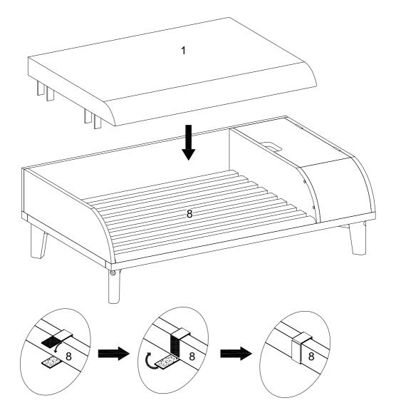
Put cushion (1) to part (8) then tighten Velcro as per diagram
