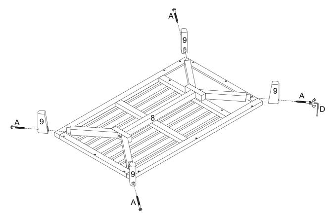
Using screw (A) attach part (9) to part (8) with Hex key (D) as per diagram.
