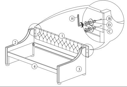
Tighten all bolts from STEP 2 using the Allen Wrench (I) that has been provided. Now only tighten bolts for STEP 3 using Allen Wrench (H). Attach Slat (7) to Front Rail (4) and Back Rail (5) by unrolling and securing with 4 Wood Screws (F) 2 per each side. Tighten all screws using philips head screwdriver (not included)
