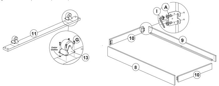
Attach Slats (11) to Front Rail (8) and Back Rail (9) using 2 Bolts (B), 2 Spring Washers (C) and 2 Flat Washers (E) on each end of each Slat (11).
