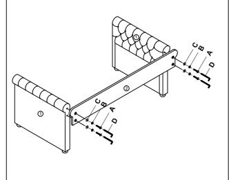
**STEP 3:** Attach Trundle Left & Right Panel (8) to Trundle Front Panel (6) and Trundle Back Panel (7), by using Allen Bolt (F), Spring Washer (G), Flat Washer (H) and Allen Key (I)
