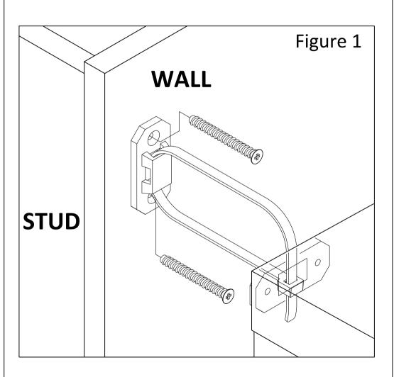
The second bracket will need to be attached horizontally to the top of furniture frame. Temporarily move furniture away from wall and place a bracket near top of frame. Mark and drill holes for screws with a 3/32" drill bit. Attach bracket to furniture piece with the two 3/4" screws. (Figure 2)
