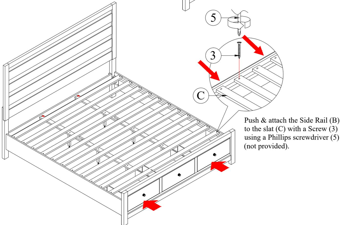
Push & attach the Side Rail (B) to the slat (C) with a Screw (3) using a Phillips screwdriver (5) (not provided).
