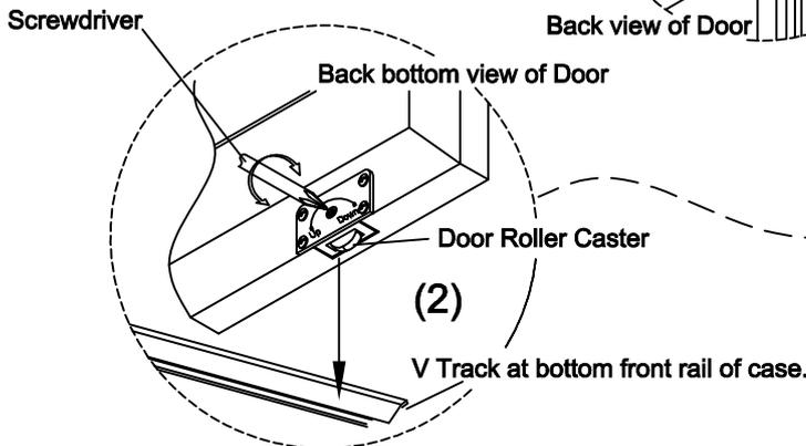
**(2) :** Place the Door Rollers at the bottom edge of door into the lower V-Track at front bottom rail of case. Make sure that both 2 Rollers stand on the V-Track, then push in the top part of door so that the top Latches of door are ready at the position of the upper U-Track at the front top rail of case.
