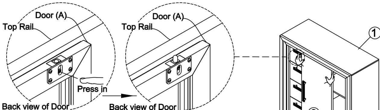
**(3) :** Use your forefingers to press in the buttons at the side of the Latches so that the Latches go up into the U-Track.
