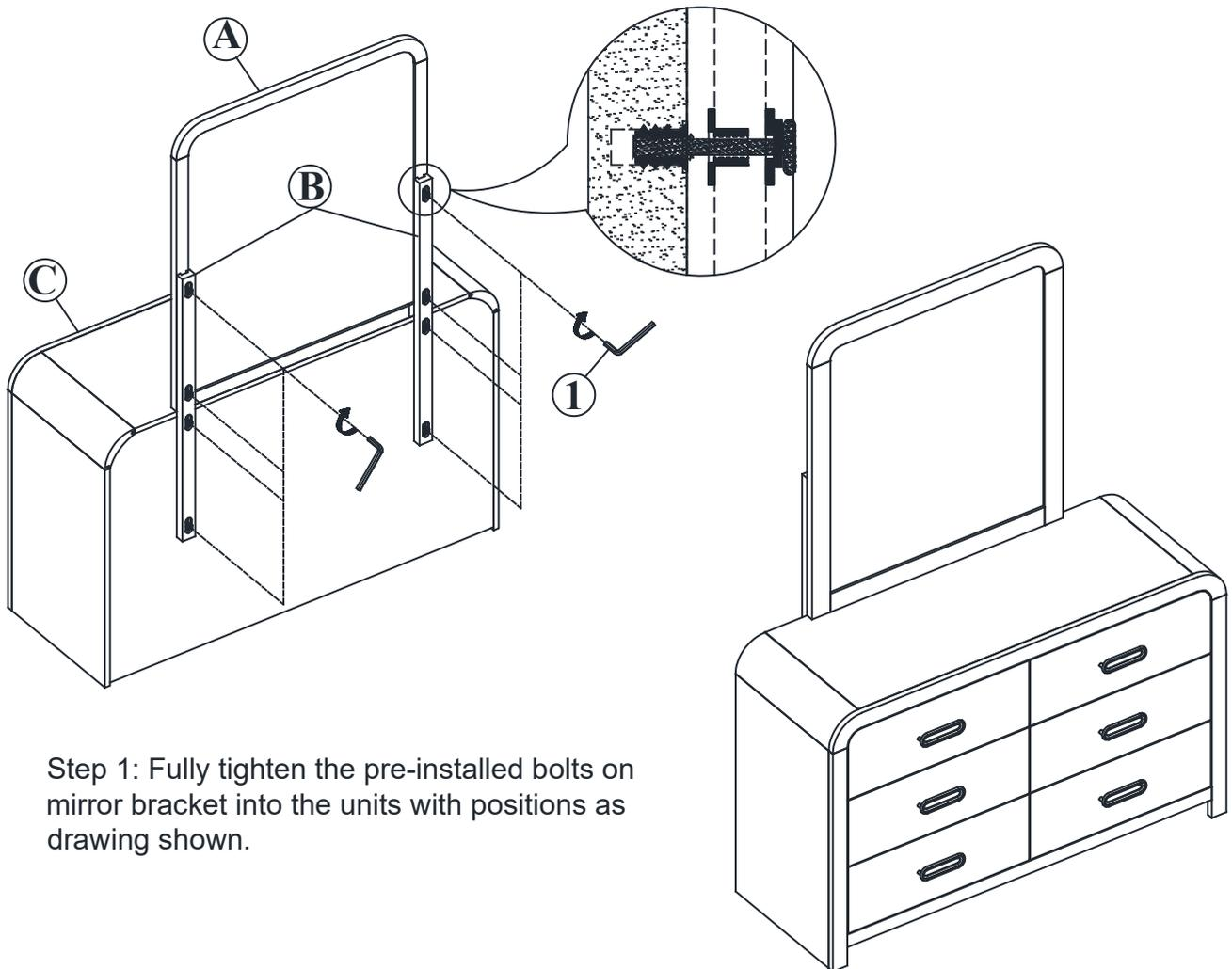
Step 1: Fully tighten the pre-installed bolts on mirror bracket into the units with positions as drawing shown.
