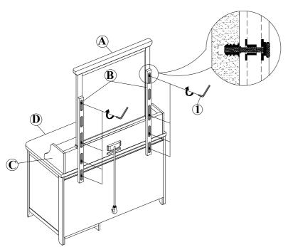
Step 1: Fully tighten the pre-installed bolts on mirror bracket into the units with positions as drawing shown.
