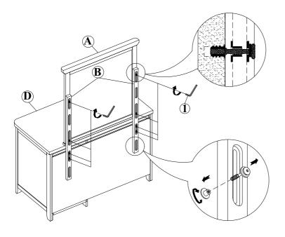
Step 1: Unbolt a pre-installed bolt on mirror bracket and then install it again as drawing shown.
