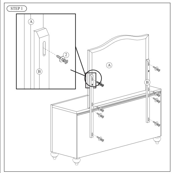
Place Mirror (A) on the top of Dresser. Align mirror to the center of the dresser and secure with 2 JCBC Bolts (2) into the dresser and 2 JCBC Bolts (2) into the mirror. Tighten bolts with Allen Wrench (1) provided.
