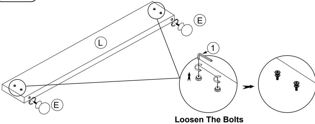
Secure the Bun foot (E) to the Footboard (L) by screwing into place. Loosen pre-assembled bolts from the Footboard (L) using the provided Allen key (1).
