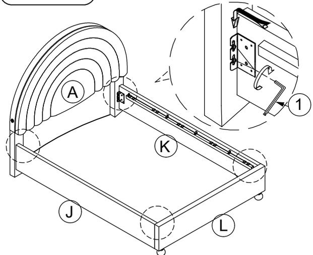
Attach the Side Rail (J) and (K) to the Headboard (A) and Footboard (L). Tighten the bolts using the Allen Key (1) provided.
