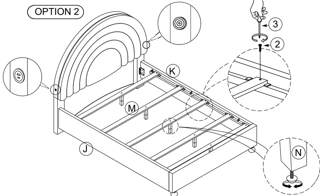
Tighten Screws (2) to the Slats (M) and Side Rail (J),(K) with Philips Screwdriver (3) (not provided).
