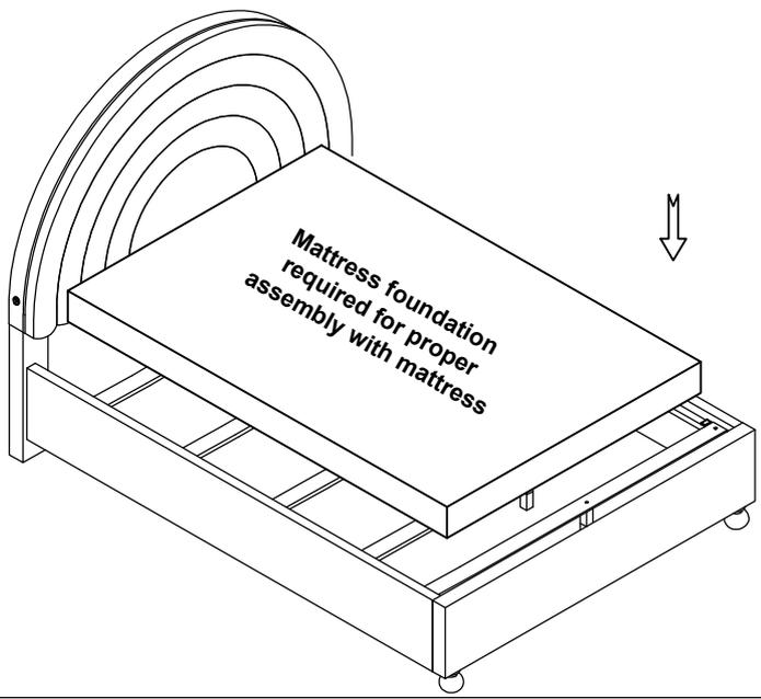
A mattress foundation is required for proper assembly with mattress. Place the mattress foundation (not provided) on top of the slats
