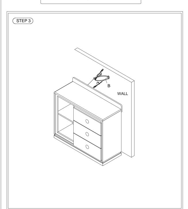
Install anti-tip kit (B) by following the assembly instructions that come in the anti tip-kit package.
