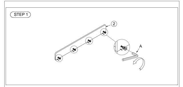
Loosen the bolts from the top back panel and attach to the case
