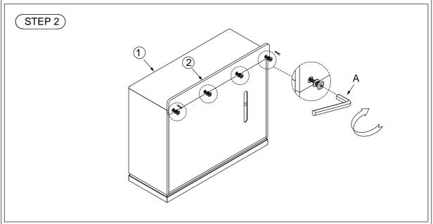
Attach the Top Back Panel (2) to the Collector Case (1). Secure with Allen Bolts, Spring Washer and Flat Washer. Tighten bolts using Allen Key (A) provided.
