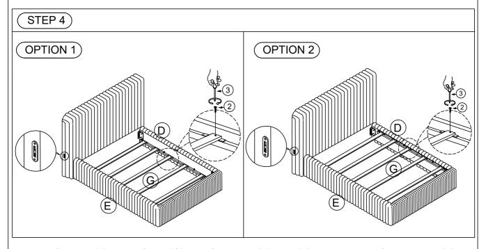
Tighten Screws (2) to the Slats (G) and Side Rail (D) and (E) using Philips Screwdriver (3) (not provided).
