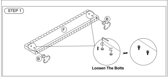
Secure the Bun foot (B) to the Footboard (F) by screwing into place. Loosen pre-assembled bolts from the Footboard (H) using the provided Allen key (1) to attach the side rails.
