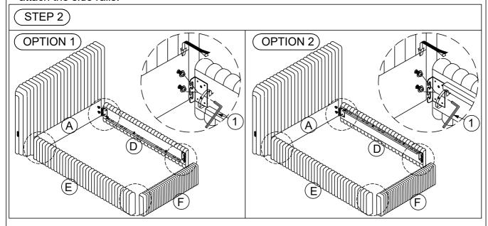
Attach the Side Rail (D) and (E) to the Headboard (A) and Footboard (F). Tighten all the bolts using the Allen Key (1) provided.
