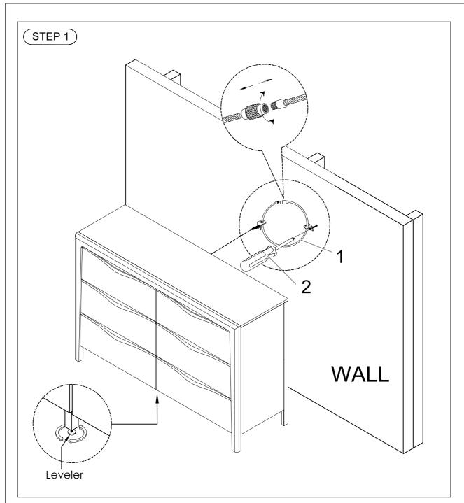
Install Tipping Restraint (1) (Customer to Assemble) with a Phillips Screwdriver (2) (Not provided) by following the assembly instructions that come in the Tipping Restraint package.
