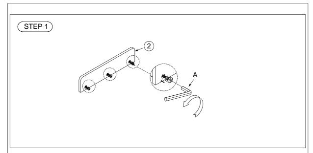
Loosen the bolts from the top back panel and attach to the nightstand
