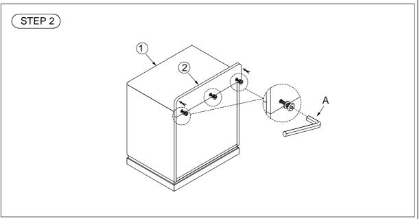
Attach the Top Back Panel (2) to the Nightstand (1). Secure with Allen Bolts, Spring Washer and Flat Washer. Tighten bolts using Allen Key (A) provided.
