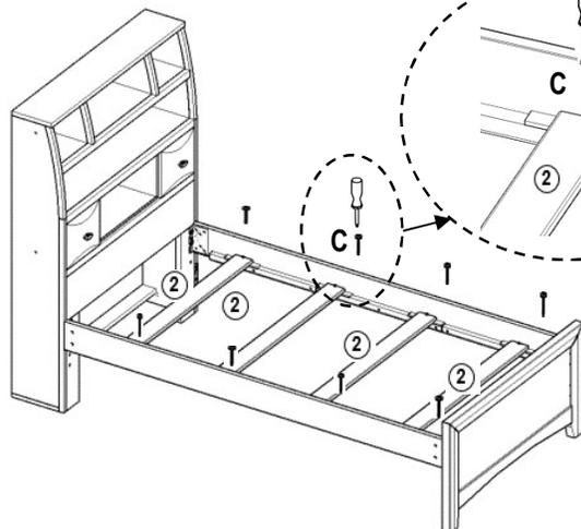
Install slats, one on each space between the small blocks,
