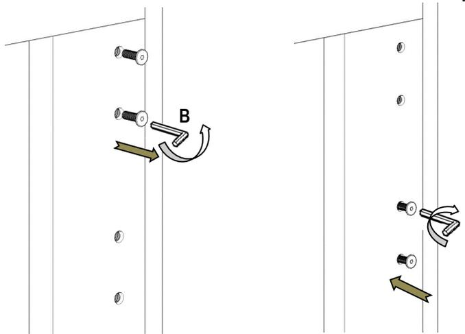
Remove bolts from top setting then install in the lower setting, do not tighten, allow 1/4" space between post and bolt head, repeat for all posts.
