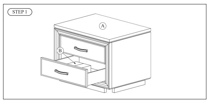
Begin assembly by removing Bunn Feet (B) from bottom of drawer of Night Stand (A).
