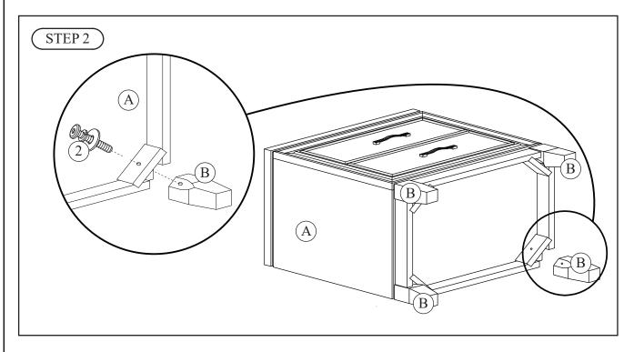
Secure Bunn Feet (B) to Night Stand (A) using 1 JCBC (2) per foot. Tighten bolts using Allen Wrench (1) provided. The assembly is now complete.
