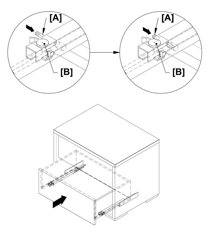
If a drawer does not close properly, or get's stuck, the most likely cause is that the drawer came of the "glide".
