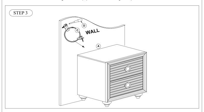
To prevent the Night Stand (A) from tipping, mount one side of the Tipping Restraint (C) to the backside of the Night Stand (A) and the other side to the wall.
