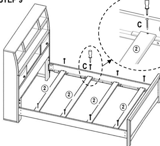
Install slats, one on each space between the small blocks, then fasten with 1 1/4" screws.
