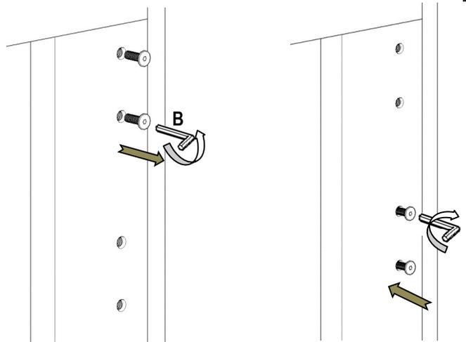
Remove bolts from top setting then install in the lower setting, do not tighten, allow 1/4" space between post and bolt head, repeat for all posts
