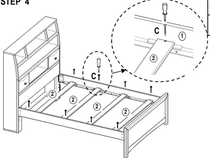
Install slats, one on each space between the small blocks,
