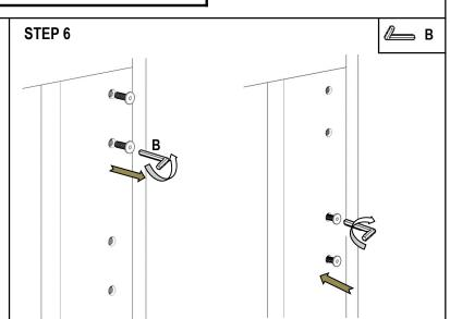
Remove bolts from top setting then install in the lower setting, do not ighten, allow 1/4" space between post and bolt head, repeat for all posts
