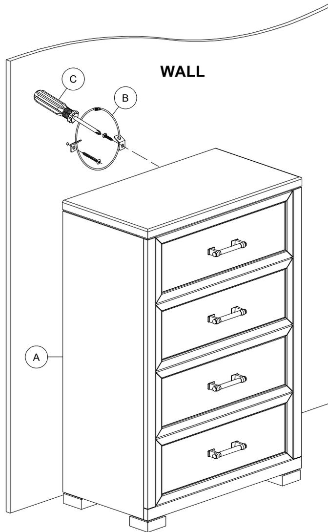
To prevent the Chest (A) from tipping, mount one side of the Tipping Restraint (B) to the backside of the Chest (A) and the other side to the wall.
