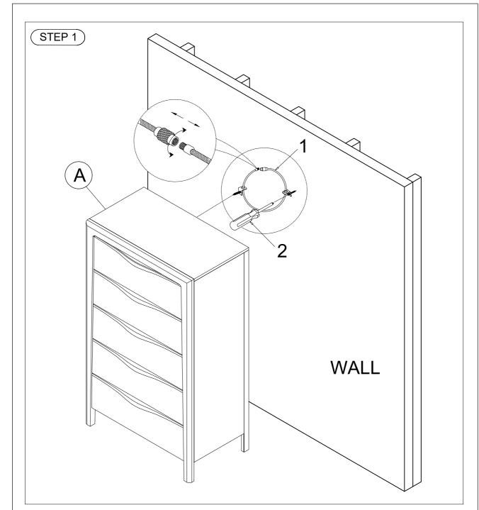
Install Tipping Restraint (1) (Customer to Assemble) with a Phillips Screwdriver (2) (Not provided) by following the assembly instructions that come in the Tipping Restraint package.
