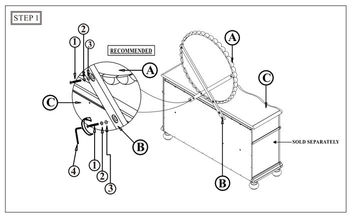
Attach Mirror Bracket (B) to Dresser (C) and Round Mirror (A) using Allen Key 4 x 60 mm (4), Lock Washer M6 x 11 x 2 mm (2), Flat Washer M6 x 16 x 1 mm (3), and Bolt M6 x 1 x 50 mm (1).
