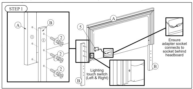
Attach the legs (B) to the Headboard (A) follow by Notification Label of 1 to 1 and 2 to 2. Secure with JCBC Bolts (2). Tighten bolts using Allen Wrench (1) provided.
