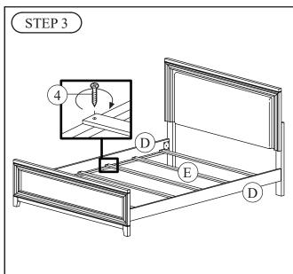
Attach Slats (E) to Side Rails (D) using Wood Screws (4). Tighten screws with Philips head screwdriver (not included).
