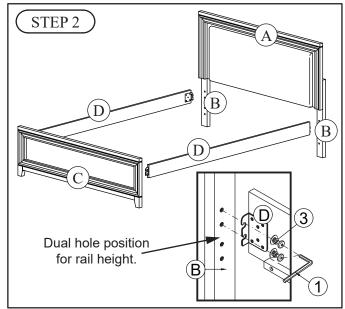
Attach the Siderails (D) to the Headboard Legs (B) by using JCBB bolts (3). Tighten bolts using Allen Wrench (1) provided. Repeat step for Footboard (C).
