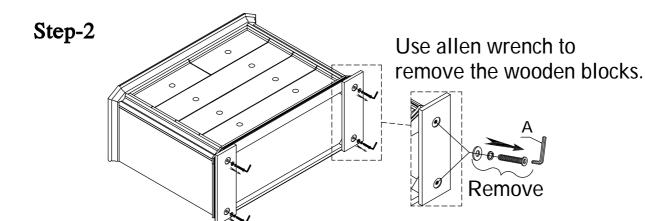
Remove all wooden blocks from the bottom of the case piece before assembling!
