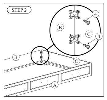
Tighten with Hinges Screw(4).
