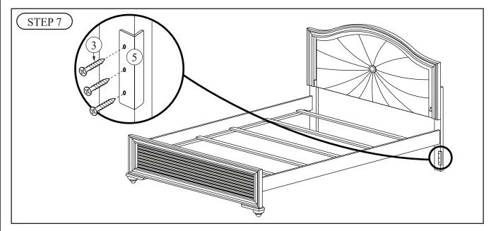
Attach Protectors (5) to the side of the footboard and headboard legs. Secure with 3 Screws (3) each. The Trundle can now be slide safely under the bed.
