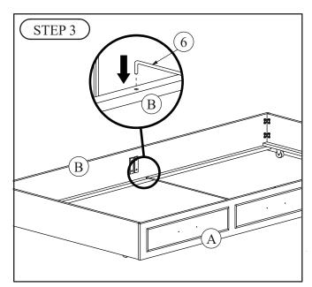
Attach the Metal Bar (6) to the Front Panel (A) & Back Panel (B).
