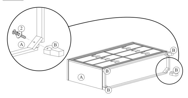
Secure Bun Feet (B) to Dresser (A) using 1 JCBC Bolt (2) per feet. Tighten bolts using Allen Wrench (1) provided. The assembly is now complete.
