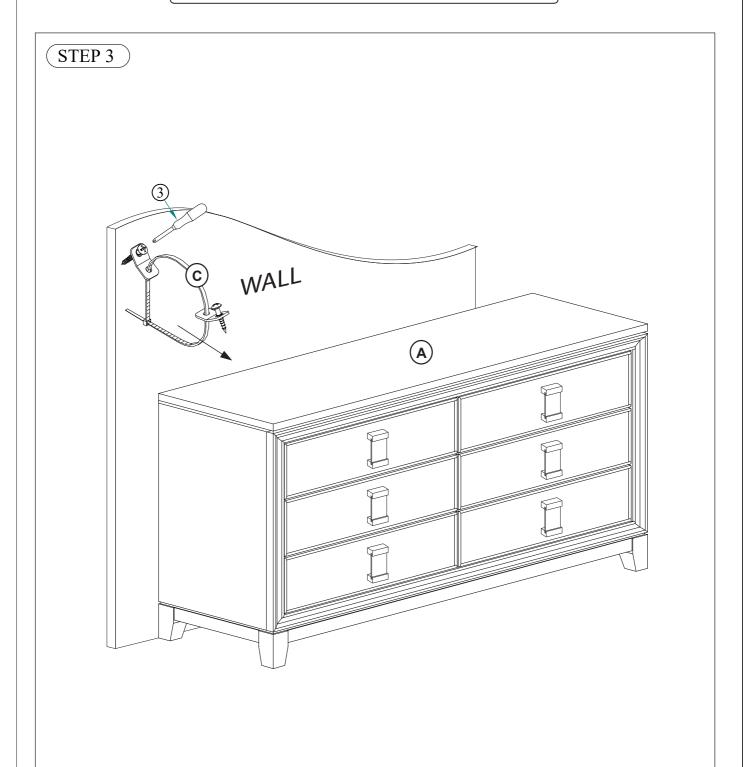
To prevent the Dresser (A) from tipping, mount 1 side of the Tipping Restraint (C) to the backside of the Dresser (A) and the other side to the wall. Tighten using Philips Head Screwdriver (not provided).
