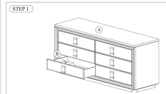
Begin assembly by removing Bun Feet (B) from bottom drawer of Dresser (A).
