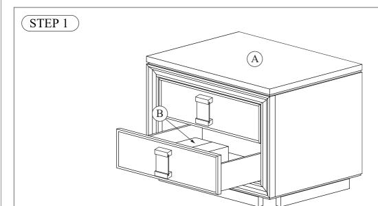
Begin assembly by removing Bun Feet (B) from bottom drawer of Night Stand (A).
