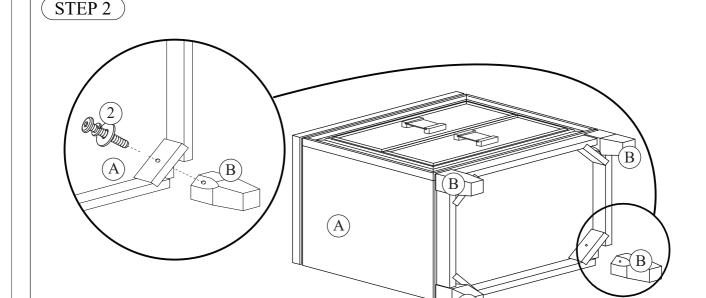
Secure Bun Feet (B) to Night Stand (A) using 1 JCBC Bolt (2) per feet. Tighten bolts using Allen Wrench (1) provided. The assembly is now complete.
