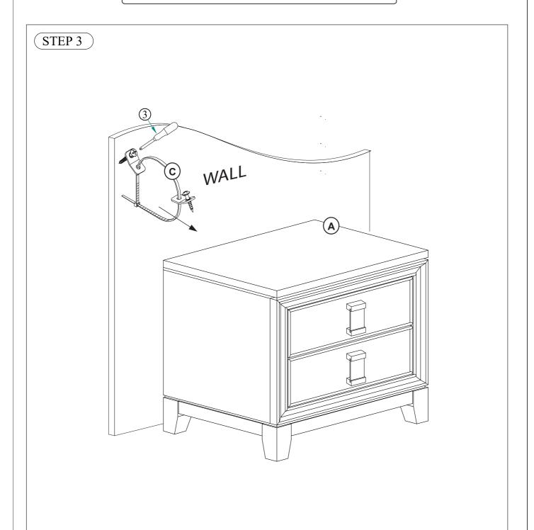
To prevent the Night Stand (A) from tipping, mount 1 side of the Tipping Restraint (C) to the backside of the Night Stand (A) and the other side to the wall. Tighten using Philips Head Screwdriver (not provided).
