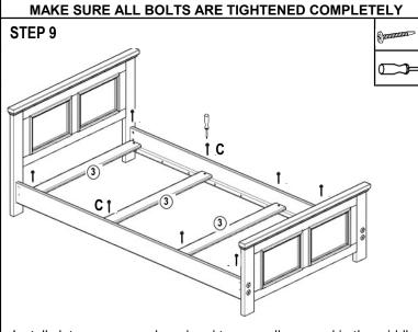
Install slats, one on each end and two equally spaced in the middle, then fasten with 1 1/4" screws.
