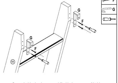
Screw ladder hooks to pre-drilled holes on top of ladder.
